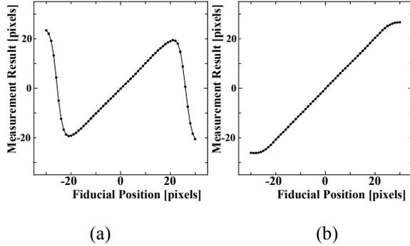
Figure 8: Positional characteristics of fiducials in the x axis. (a) shows the characteristics of Figure 7(a). (b) shows the characteristics of Figure 7(b).
