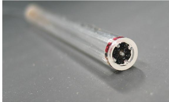
Figure 13: Sensor head of the pen device.
