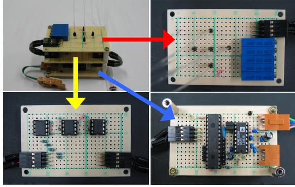
Figure 16: Electrical circuit of the receiver.
