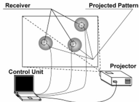
Figure 2: System configuration
