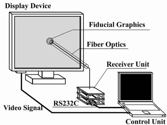
Figure 14: System configuration of the pen type receiver.
