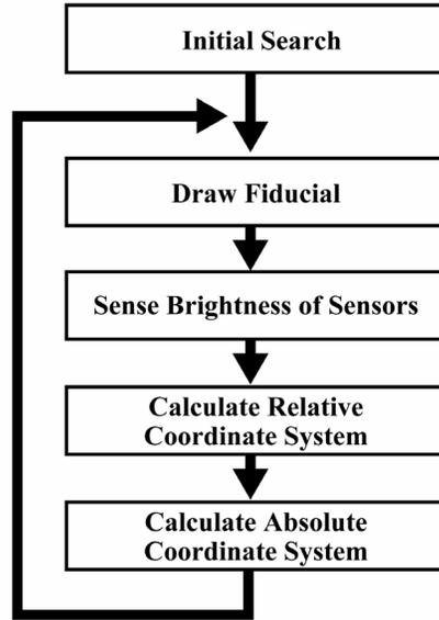
Figure 11: Tracking Process
