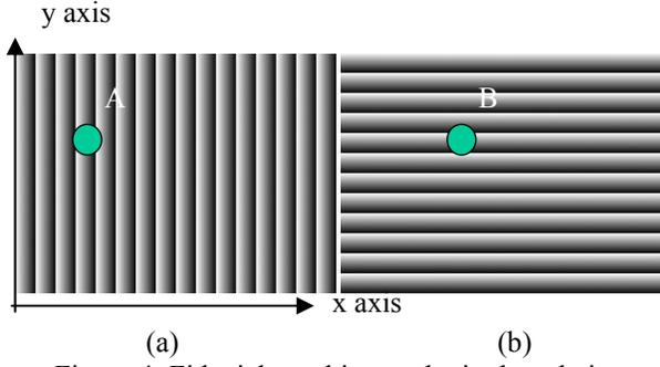
Figure 4: Fiducial graphics to obtain the relative position of the sensor.
