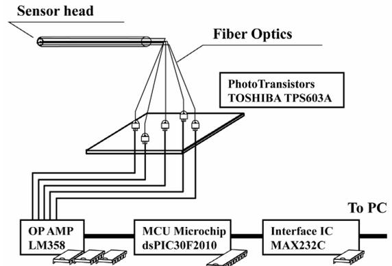
Figure 15: Block diagram of the pen type receiver.
