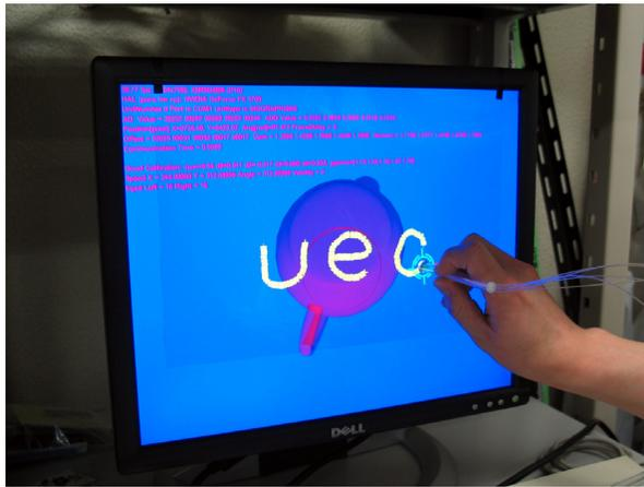
Figure 17: Snapshot of the pen type receiver tracking.
